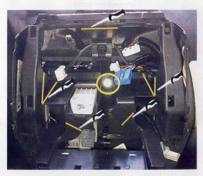
CUT OEM DASHBOARD IN THE POSITIONS SHOWN IN THE PICTURE, UNSCREW THE CENTRAL SCREW POSITIONED ON THE BOTTOM, AND REMOVE THIS PART TO ALLOW THE FIXING OF THE AFTERMARKET RADIO.
