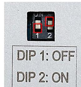
**After each Dip-switch-change a power-reset of the Can-box has to be performed!**
