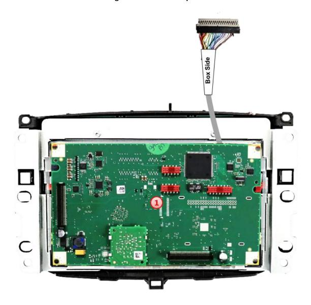
Bring the previously set aside original PCB in position with its 4 screw holes to the thread sockets of the exchange metal plate-2 and restore the connection of the plug contacts.
