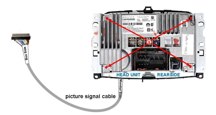
Carefully lead the monitor's rear part into the exchange metal plate-2, restore the connection of the plug contacts and fix it to the monitor's housing by using the 4 longer screws.
