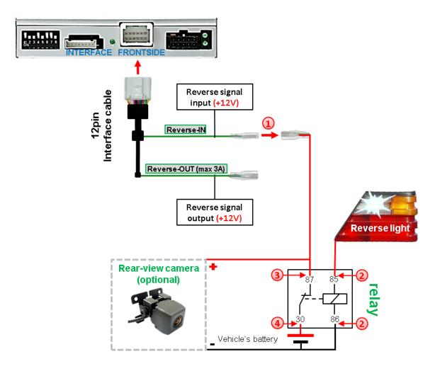
Disconnect the green cable's pre-connected male- and female connectors of the 20pin cable and connect the green input cable "Reverse-IN" to the output connector (87) of the relay.
