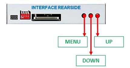
The picture settings can be adjusted by the 3 buttons on the video-interface. Press the **MENU** button to open the OSD settings menu. To switch to the next menu item, pressing **UP** and **DOWN** will change the selected value. The buttons are embedded in the housing to avoid accidental changes during or after installation. The picture settings have to be done separately, AV1 and AV2 while the corresponding input is selected and visible on the monitor.
