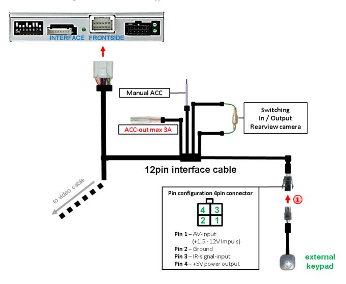
Connect the keypad's female 4pin connector to the video-interface's male 4pin connector.
