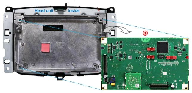
(1) Carefully plug the PCB out of the original metal housing parts and lay it aside.
