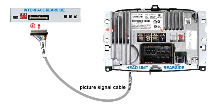
Connect the picture signal cable's beige coloured female 20pin connector, which is lead out from the head unit, to the male 20pin connector of the video-interface.
