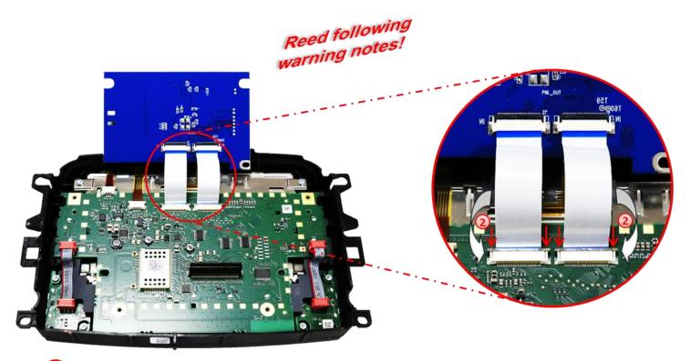
2 Bring the daughter PCB in position and connect it's preconnected ribbon cables "IN" to the previously become free ribbon cable bases of the original PCB. Carefully fix the ribbon cables by pushing the locks in direction of the arrows as shown in the illustration.
