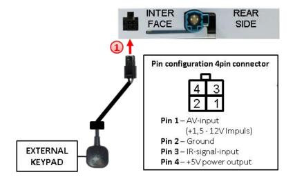
Connect the 4pin female connector of the external keypad to the male 4pin connector of the video interface.
