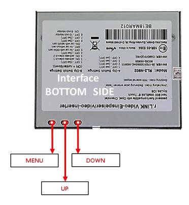
The picture settings are adjusted by the 3 buttons on the video-interface. Press the MENU button to open the OSD settings menu or to switch to the next menu item. Press UP and DOWN changes the selected value. The buttons are embedded in the housing to avoid accidental changes during or after the installation. Picture settings have to be done separately for AV1, AV2 and CAMERA-IN while the corresponding input is selected and visible on the monitor.
