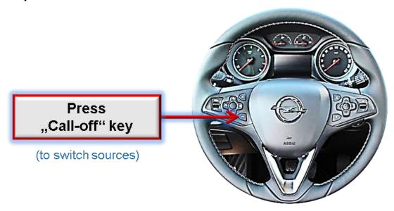
Switching the video sources can be done by pressing the vehicle's "Call-off" button.
