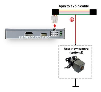
Additionally, the +12V (max. 500mA) power supply for the rear-view camera can be taken from the green wire of the 6pin to 12pin cable.
