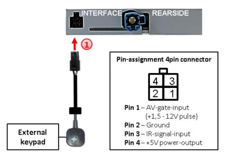
Connect the 4pin female connector of the external keypad to the male 4pin connector of the video interface.
