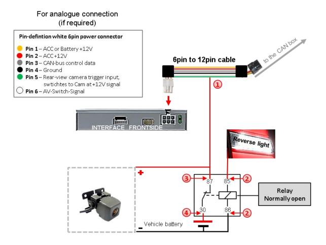
Connect the green cable of the 6pin to 12pin cable to the output connector (87) of the relay.
