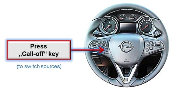
Switching the video sources can be done by pressing the vehicle's **"Call-off"** button.
