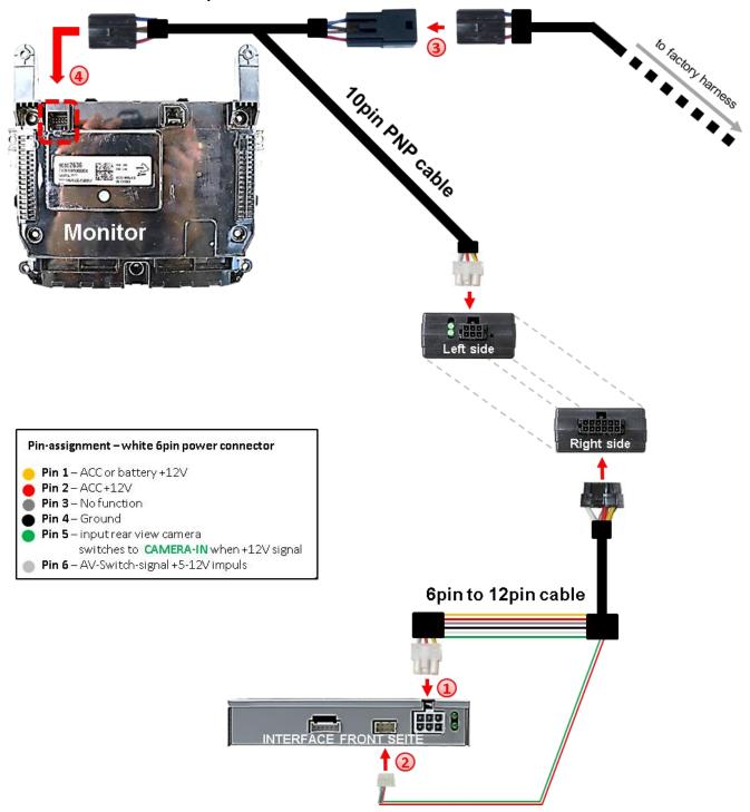
Connect the female 6pin connector of the 6 to 12pin cable to the 6pin connector of the video interface.
