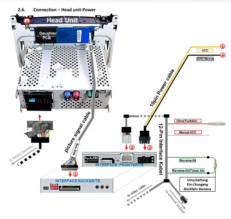
Connect the 20pin picture signal cable's female 20pin connector to the male 20pin connector of the video-interface.
