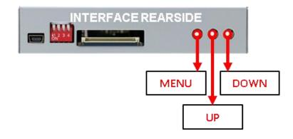
The picture settings adjustment can be done by the 3 buttons of the video-interface. Press the **MENU** button to open the OSD settings menu. To switch to the next menu item, pressing **UP** and **DOWN** will change the selected value. The buttons are embedded in the housing to avoid accidental changes during or after installation. The picture settings have to be done separately for AV1 and AV2 while the corresponding input is selected and visible on the monitor.
