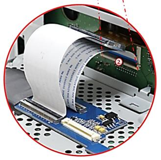
Connect the daughter PCB's pre-assembeled inner 40pin ribbon cable to the previously become free ribbon cable base of the monitor mainboard.
