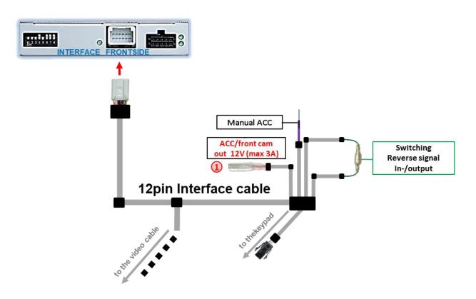
The red power supply output ACC/front cam out 12V (max 3A) can be used to power an external source and has a different assignment depending on the position of dip switch 1 (of the black 8 dips):
