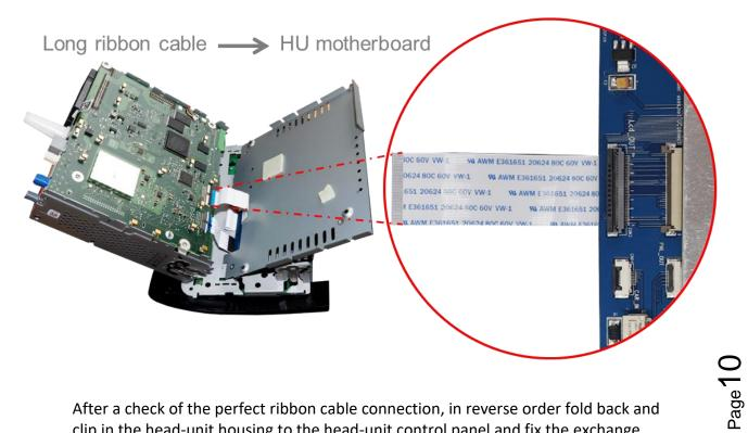
After a check of the perfect ribbon cable connection, in reverse order fold back and clip in the head-unit housing to the head-unit control panel and fix the exchange housing base plate to the head-unit's housing.
