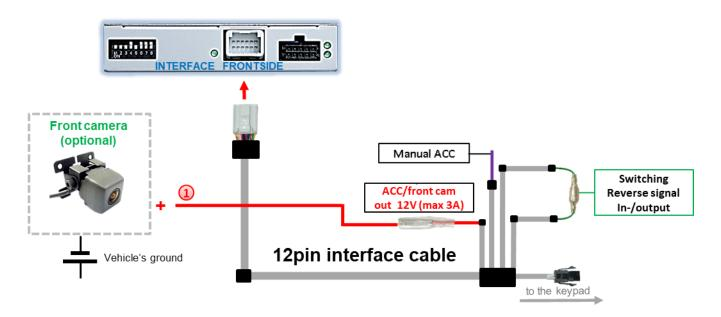
The red power supply output ACC/front cam out 12V (max 3A) can be used to power a front camera. If Dip 1 is set to ON (black 8 dips), the power supply output gives +12V (max 3A) when reverse gear is engaged incl. 10 seconds delay after reverse gear is disengaged.
