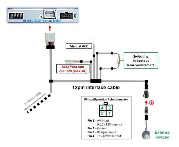
Connect the keypad's female 4pin connector to the 12pin interface cable's male 4pin connector.
