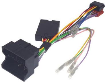
This interface provides steering wheel control commands to the new head unit and gives CAN signal outputs; speed pulse (pink wire), illumination (orange wire), reverse gear (purple wire) and hand brake (green wire). It also allows the PDC and climate control information to be displayed on the car's white display on the instrument cluster. This interface also has amplifier turn on and control features.
