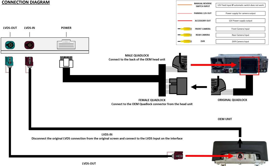
Connect the NEW LVDS cable from the LVDS output on interface to the LVDS connection on the Original screen
