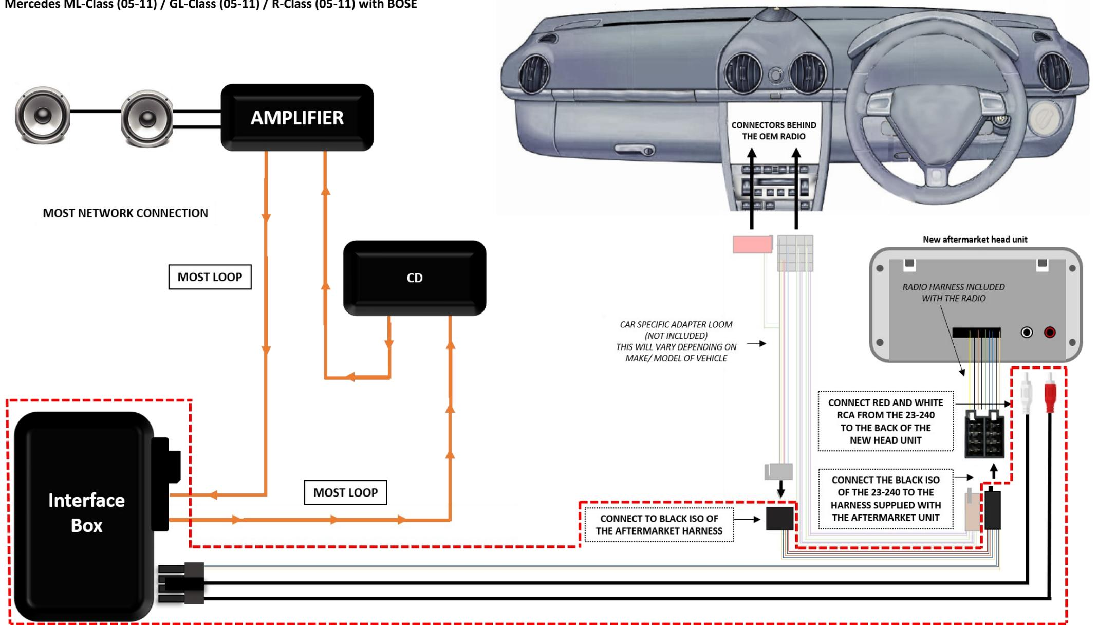
*\*The Red Border indicates the 23-240 components and where to make necessary connections*
