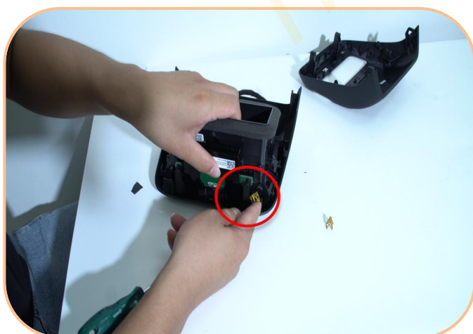
11. Install the clips onto the screen panel
