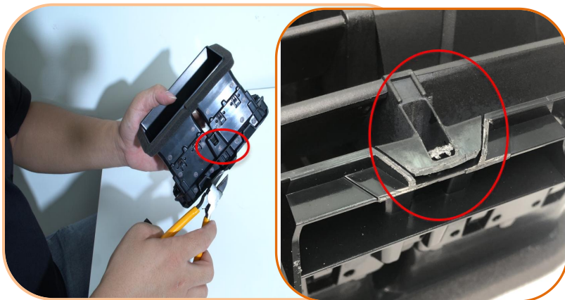
8. Cut off the middle clip at the top of the A/C outlet.
