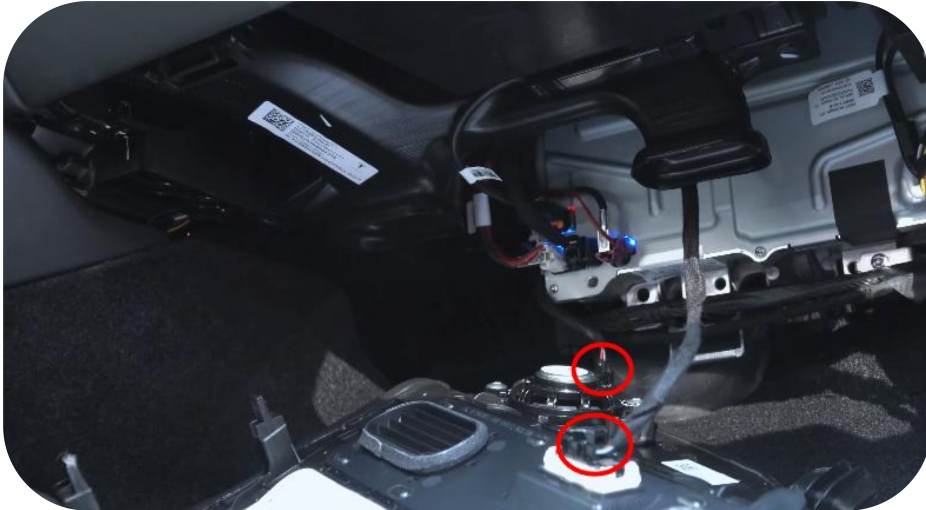
10. Unplug the footrest lamp plug and speaker plug on the decorative panel
